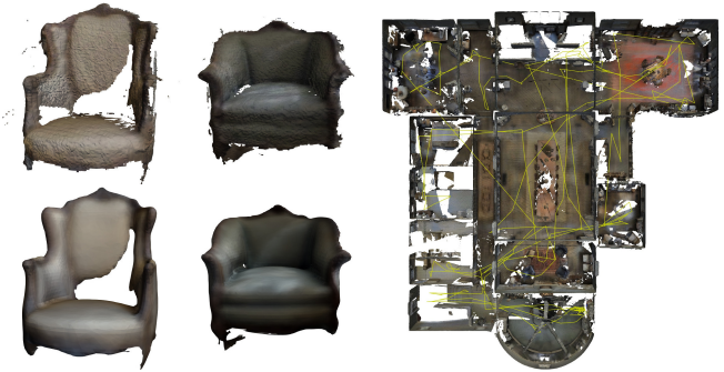
Fig. 1. Objects reconstructed using our method [Top left] and their corresponding ground-truth meshes provided by the Matterport3D dataset [9] [Bottom left]. Top-down view of 3D reconstruction after exploration, and MAV path in yellow [Right].
